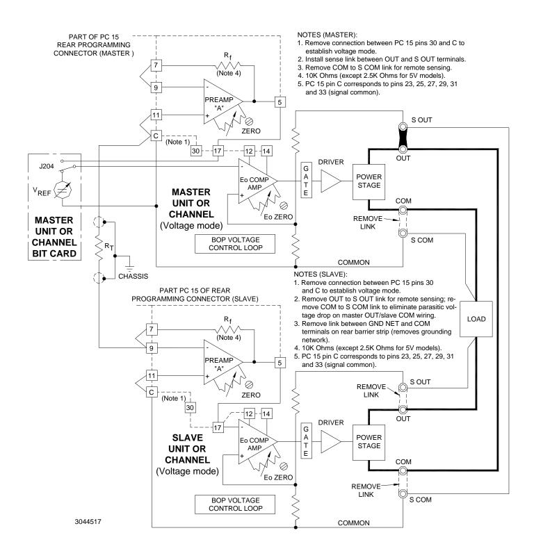
FIGURE 5. SERIES CONNECTION, VOLTAGE MODE (SHOWN), MASTER/SLAVE WITH DIGITAL CONTROL OF MASTER, REMOTE ERROR SENSING, SLAVE BIT CARD DISABLED (APPLIES TO BOP 2X-DE CHANNELS)
