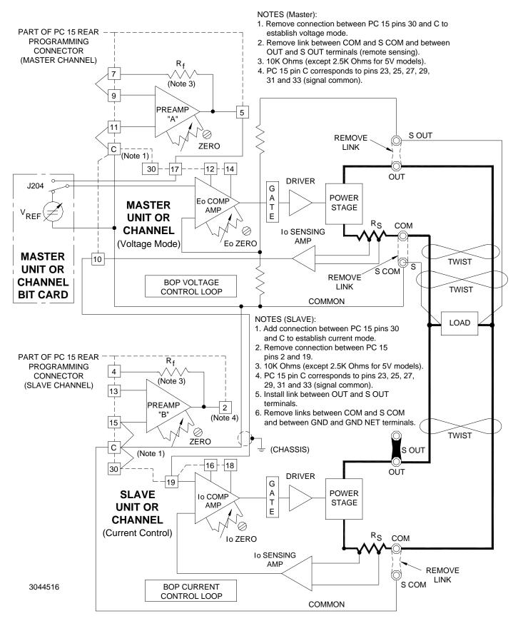
FIGURE 4. PARALLEL CONNECTION, VOLTAGE MODE (SHOWN) MASTER/SLAVE WITH DIGITAL CONTROL OF MASTER, REMOTE ERROR SENSING, SLAVE BIT CARD DISABLED (APPLIES TO BOP 2X-DE CHANNELS)
